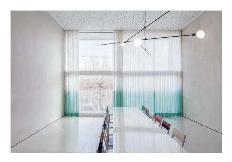
"I always liked to play with counterweights to create movement and tension in my products. With the Still lamp, the rod of metal that creates the balance has the same diameter as the tube welcoming the cable. Screwed together, they create a perfect line and allow easy packing when separated."
