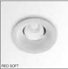
REO SOFT 2700-1800K CRI > 90 / 760lm (9,5W) REFLECTOR 40°
