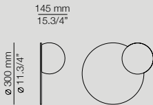
CIR_3702 LED 10W (2700K) Typ* 870 lumens Dimmable triac *Optional dimming available
